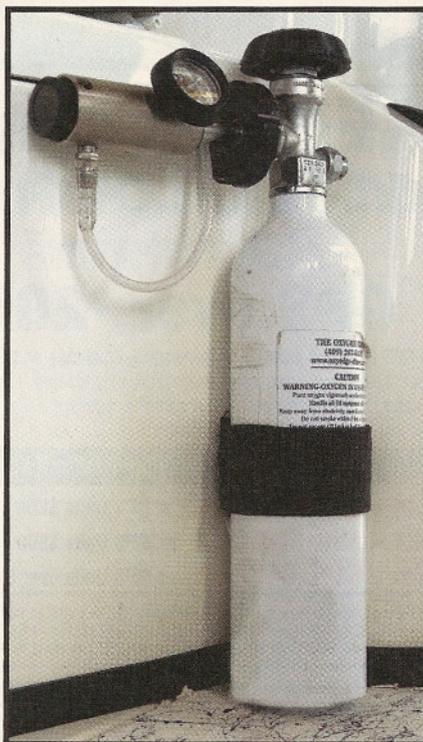
**Compressed oxygen tank is firmly secured near the livewell it serves. Using one of these systems is a big responsibility for the skipper.**
